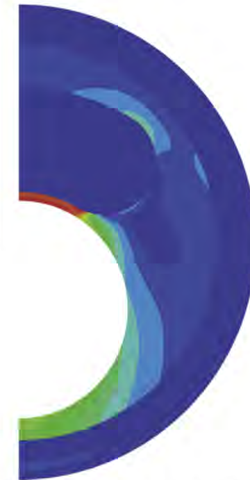
Figure 3 Contour map of von Mises stresses in half cross-section of a plaque model with intermediate intima stiffness. The highest stresses are in the cap and the peak stress values in the midcap and shoulder region are similar.
